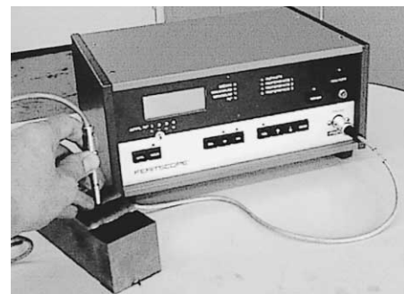
Fig. 3 - A Feritscope is most useful for measuring ferrite content of weld metals at site, because the probe is small enough to put on a small area of weld metal
